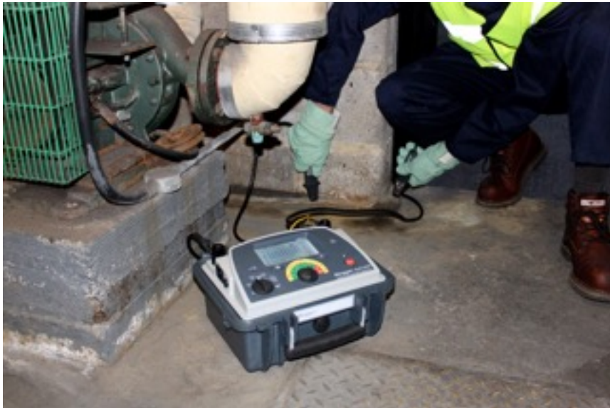
Fig16: The heavy duty DLRO10HD taking a measurement
